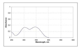
Tinuvin 234 exhibits high absorbance in the 300-400 nm region and minimal absorbance in the visible region (>400 nm) of the spectrum. The absorption maxima are at 302 nm and 343 nm (ε =16'100 l/ mol.cm) in chloroform solution.
