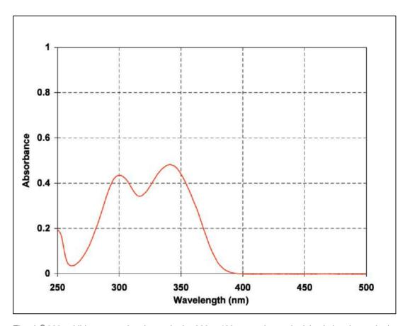
Tinuvin® 329 exhibits strong absorbance in the 300 – 400 nm region and minimal absorbance in the visible region (> 400 nm) of the spectrum. The absorption maxima are at 301 nm and 343 nm ( $\epsilon$  = 15910 l/mol·cm) in chloroform solution.
