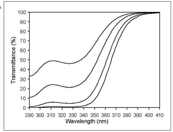
Top line: 0.001% Chimassorb® 81, corresponds to 0.25 % in a 40  $\mu$ m film Second Line: 0.002% Chimassorb® 81, corresponds to 0.50 % in a 40  $\mu$ m film Third Line: 0.004% Chimassorb® 81, corresponds to 1.00 % in a 40  $\mu$ m film Bottom Line: 0.006% Chimassorb® 81, corresponds to 1.50 % in a 40  $\mu$ m film
