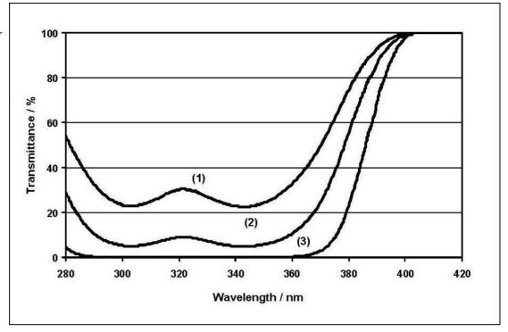
Line one: 0.003 % Tinuvin® 5050 corresponds to 0.68% active UVA in a 40  $\mu$ m film Line two: 0.005 % Tinuvin® 5050 corresponds to 1.35% active UVA in a 40  $\mu$ m film Line three: 0.014 % Tinuvin® 5050 corresponds to 3.38% active UVA in a 40  $\mu$ m film
